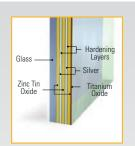
glass (coated with eight layers of high performance reflective metallic shields) and one pane of clear glass. Complete with the MAXEdge™ spacer system and two chambers filled with high density krypton gas.
