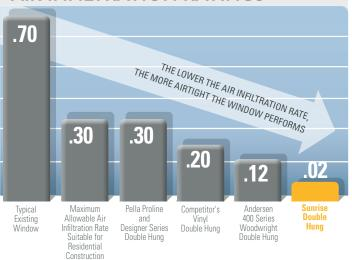
With a constant 25 mile per hour wind, this test shows how many cubic feet of air infiltrates through each square foot of the window each minute. Results are from Pella Product Guide Specification 2008, and Andersen 2009 Performance Standards. Sunrise Double Hung results from April 2016 testing.
